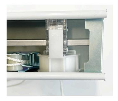
Tilter controller in a normal size blinds will be located at one of the far ends. You can identify it by looking at the shape and you will see some sort of a wheel.
