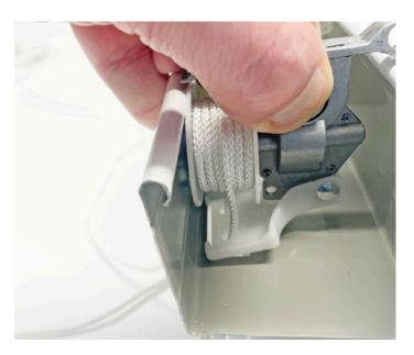
On a slight angle slot the base of the tilter into the slot.
